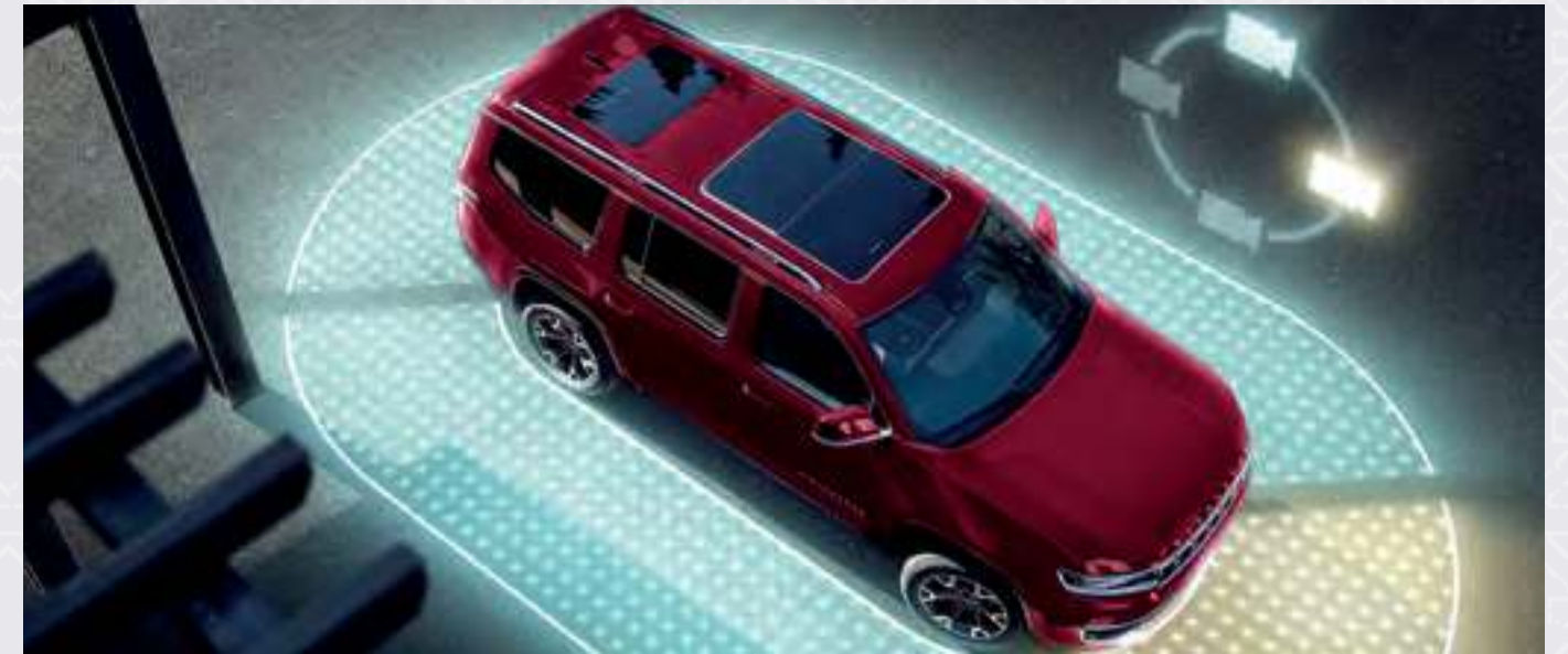
360° SURROUND-VIEW CAMERA 4 — The vehicle's entire perimeter is monitored and displayed on the Uconnect ® touchscreen, providing several views, like top view, rearview and 360-degree view, to assist the driver when maneuvering tight spaces. Standard on Grand Wagoneer and available on Wagoneer.
