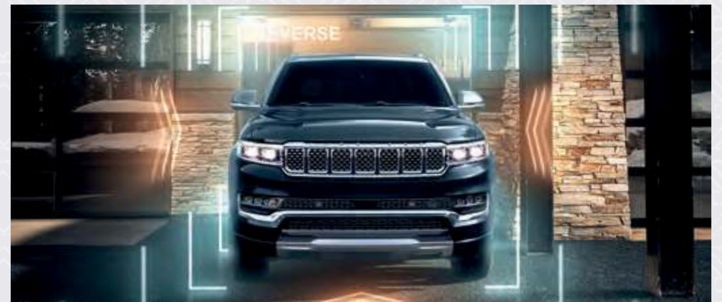
PARKSENSE ® AUTOMATED PARKING SYSTEM 6 — Ultrasonic sensors located at the vehicle's front, rear and sides help detect a parking spot. The system then automatically steers your vehicle into the detected spot while using advanced brake and throttle control. Standard exclusively on Grand Wagoneer.
