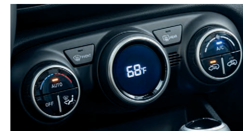
Automatic temperature control
