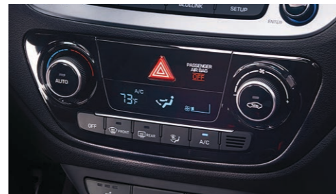
Automatic temperature control
